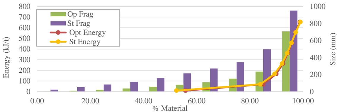
**Figure 8. Comparison of Energy and Fragmentation Distribution between two designs: Standard and Optimized**
