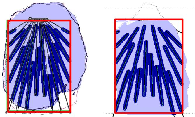
**Figure 9. Energy simulation, design and final stope geometry. Standard and optimized designs**
