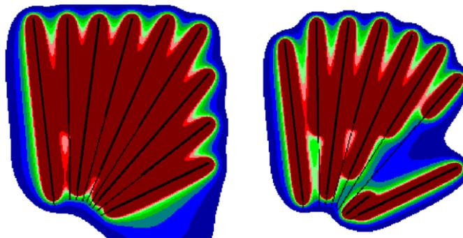
**Figure 7. Design and real explosive energy distribution**
