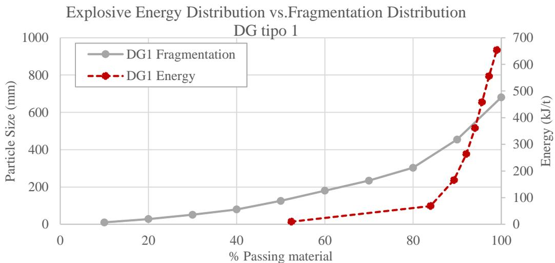
**Figure 1. Explosive Energy distribution and Fragmentation distribution of DG tipo 1 ore domain**
