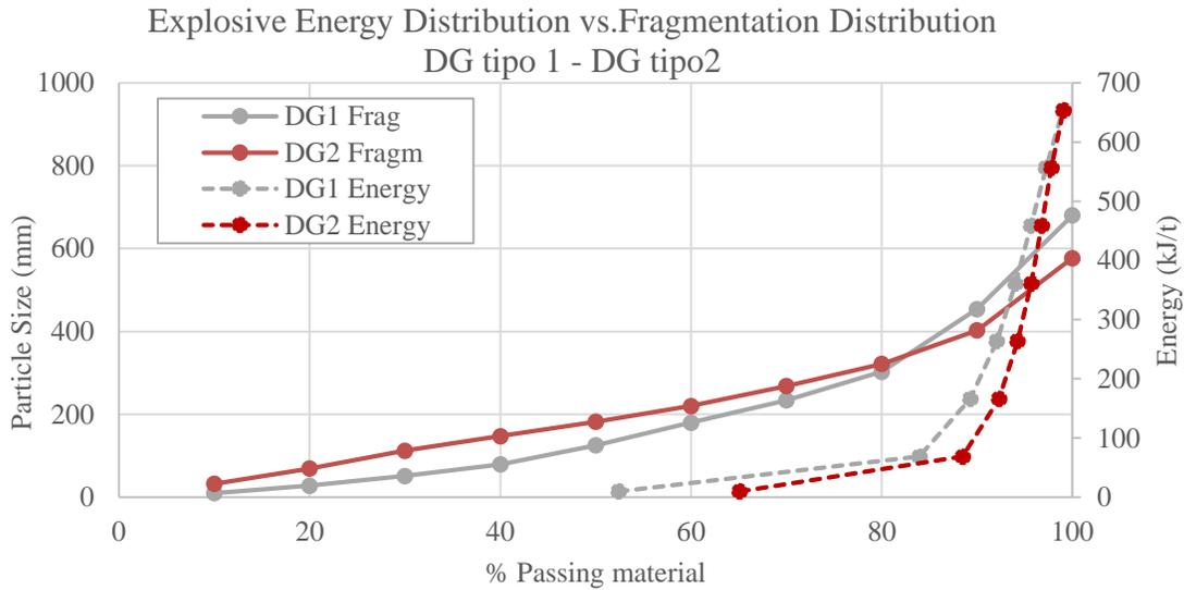
**Figure 2. Explosive Energy distribution and Fragmentation distribution of DG1 and DG2**
