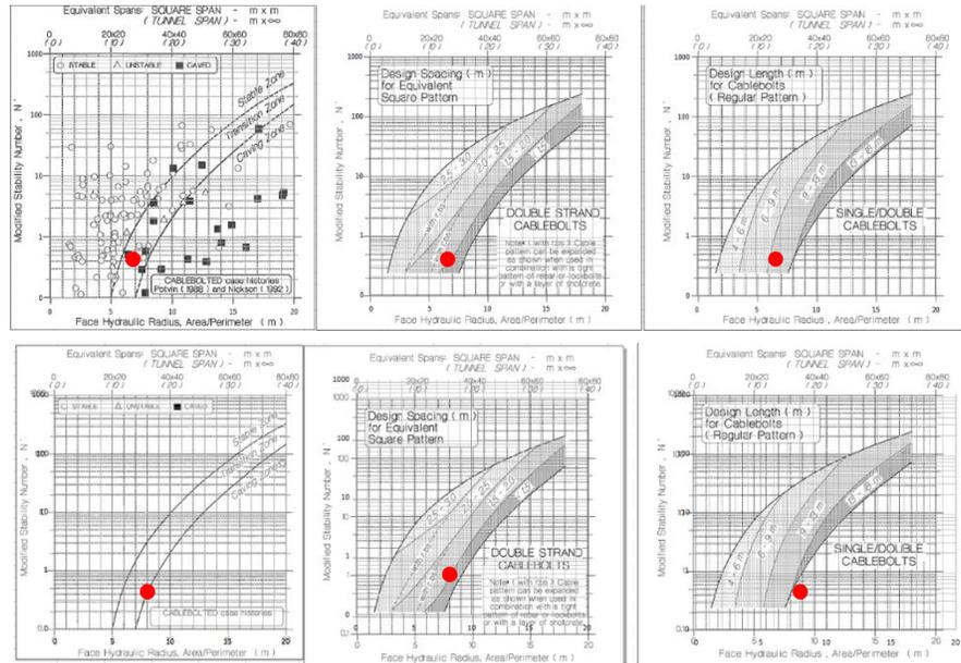
Figure 4. Theoretical HR and support (up) and Real HR and necessary support (down)
