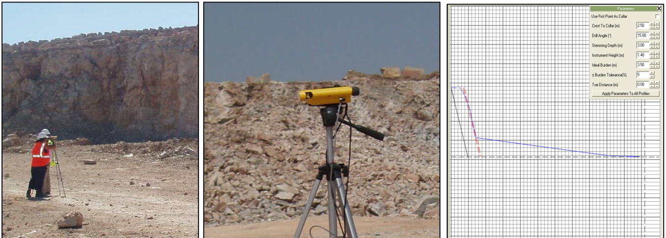
Figures 5, 6 and 7: Laser 2D profiling before drilling for positioning
